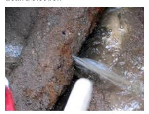
Do an overnight, or night time, test when the business is "resting" or little water is being consumed. Work out the litres per hour that goes through your meter = your leak. Multiply by 8760 and that is your annual leak. Multiply by the total cost of water and that is the cost.
